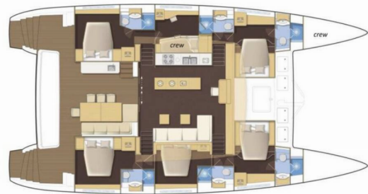
Cucine centrale, 6 cabins / Central galley, 6 cabin version
